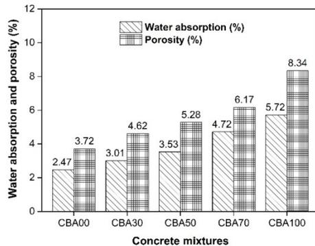
Fig. 7. WA and porosity of concretes.
