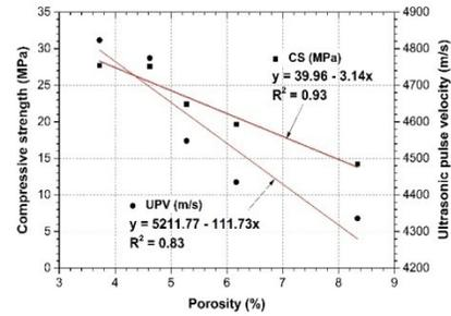
Fig. 8. The relationship between porosity and CS and UPV of concretes.
