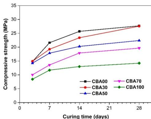
Fig. 3. Compressive strength of concretes.
